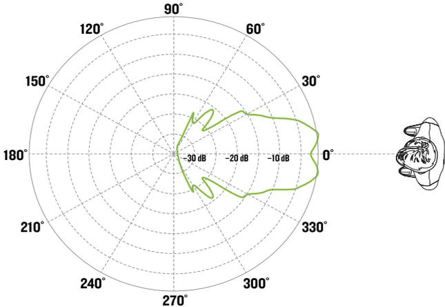
**SRT POLAR MEASUREMENTS OF VERTICAL DISPERSION (MF + HF)**
