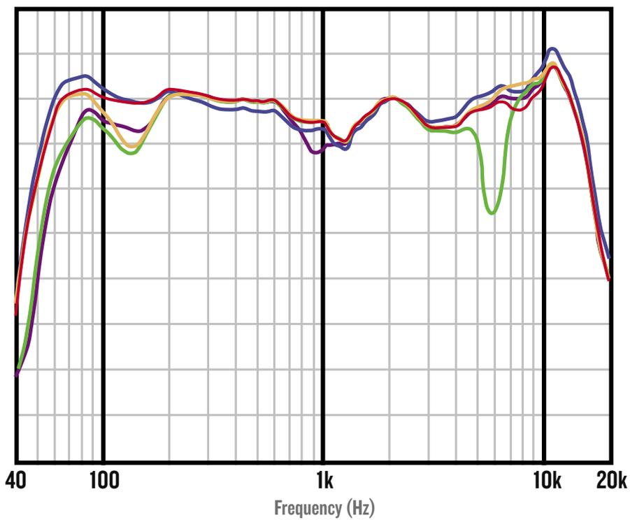
**SRT POLAR MEASUREMENTS OF HORIZONTAL DISPERSION (MF + HF)**
